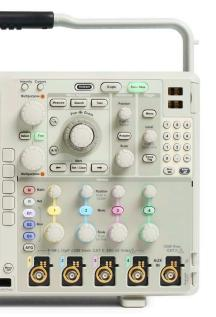
Two or four analog channels will allow you to view and compare signal timings of your multiple waveforms. Debugging a digital system with parallel data requires an additional eight or 16 digital channels (or more). A Mixed Signal Oscilloscope (MSO) adds digital timing channels, which indicate high or low states and can be displayed together as a bus waveform.
